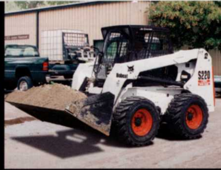
Skid-steer loading topdresser
