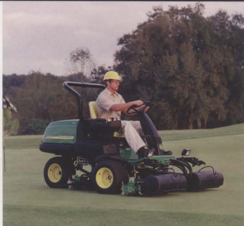
One of the most important features on John Deere's 2500 triplex riding greens mower is the patented offset cutting units, especially critical on daily cleanup passes.
