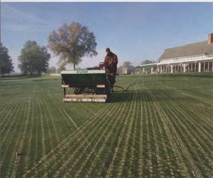
Superintendents are exploring alternatives to traditional aerification, including substituting powerful streams of water for tines via a DryJect machine.
