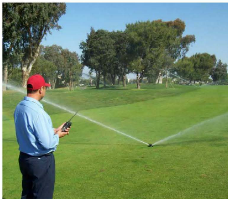
Regularly checking arc adjustment, spray pattern and pressure is a simple way to determine the efficiency of an irrigation system. Replacing faulty nozzles can be an inexpensive solution to improve distribution and reduce water consumption.
