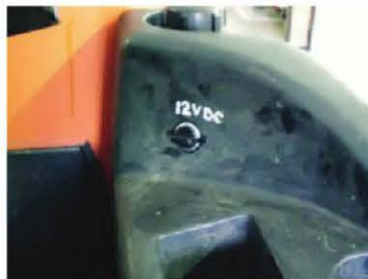
Left: A handle placed on the hood of a Jacobsen LF 3400 offers a safe place to put your hand when wrestling with the engine cover. Center: The addition of a light, a popular operator request, as well as the addition of a 12v power outlet (right).
