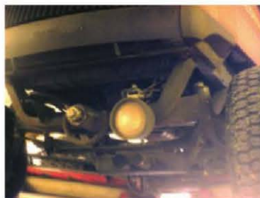
Left: A handle placed on the hood of a Jacobsen LF 3400 offers a safe place to put your hand when wrestling with the engine cover. Center: The addition of a light, a popular operator request, as well as the addition of a 12v power outlet (right).
