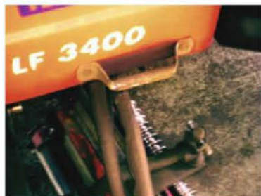
Left: A handle placed on the hood of a Jacobsen LF 3400 offers a safe place to put your hand when wrestling with the engine cover. Center: The addition of a light, a popular operator request, as well as the addition of a 12v power outlet (right).
