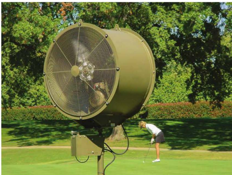
Fans can lower greens surface temperatures by as much as 10 degrees and soil temperature by 4 to 6 degrees Fahrenheit.
