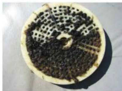
An example of bryozoa clogging a bottom filter, reducing efficiency.
