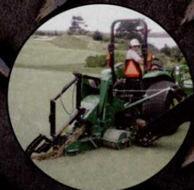
Turf Surgeon Verticuts and Collects
