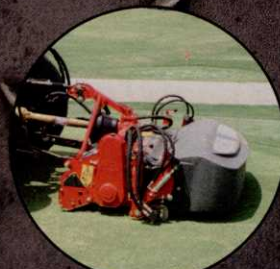
Turf Surgeon Verticuts and Collects
