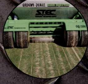
**Ground Quake Sand Injector**
