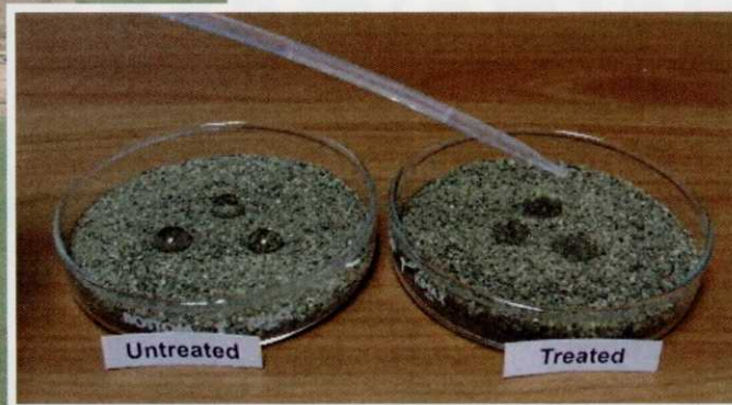
Left, localized dry spots (LDS) caused by water repellent soil. Above, an instant visual of what happens to drops of water on treated and untreated soil.
