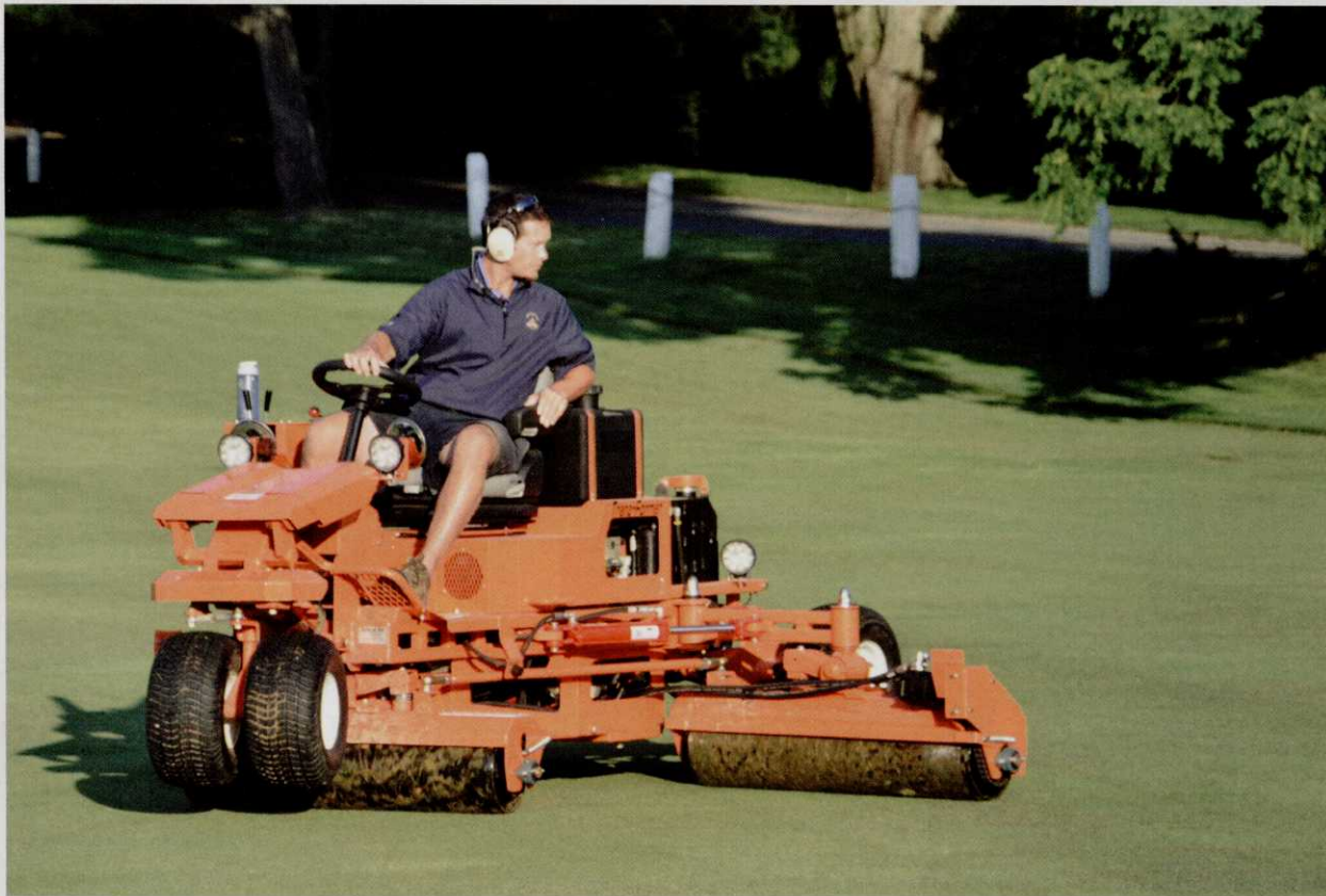
Sal Rizzo: "We built a small model and worked on the steering for what seemed to be forever. We were positive that when turning on the green there should be no damage. It took four months alone just to perfect the steering."
