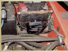
power cord. Another option is to install a CTEK Multi US 3300 battery charger that ranges in price from \$50 to \$250. The unit puts the batteries through an eight-step reconditioning process that revives dead or borderline batteries by maintaining
