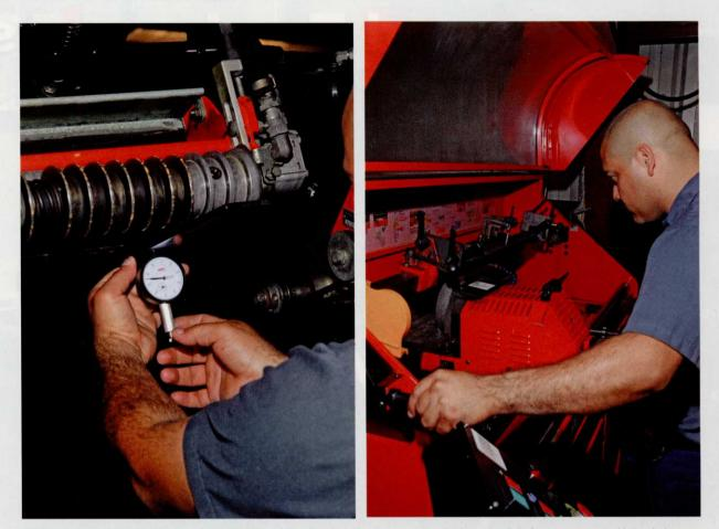
With advances in technology and materials, backlapping is taking up less time in the schedule for many crews. Not only has backlapping compound improved, high-hardness materials for reels and bedknives keep their edge longer.
