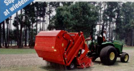
SUPER 500 Verticut and pulverize in one pass
