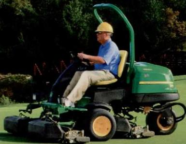
Offset cutting units – Introduced to prevent “triplex ring”.
