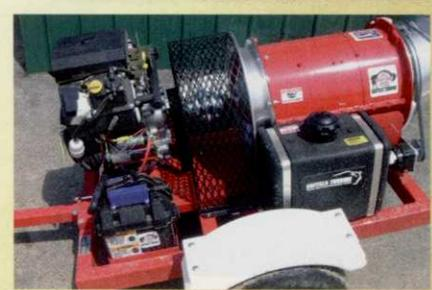
The engine battery is used to change the blower nozzle direction, as it is hooked up to the alternator on the tow vehicle with pig tails to keep the battery charged at all times. The blower RPM's are changed as needed by changing the ground speed of the tow vehicle with the throttle lock when desired. The blower is significantly quieter than when it had an engine and it saved the club over \$2,000 for a new engine. The used real motor cost \$65 and it took about eight hours to build.
