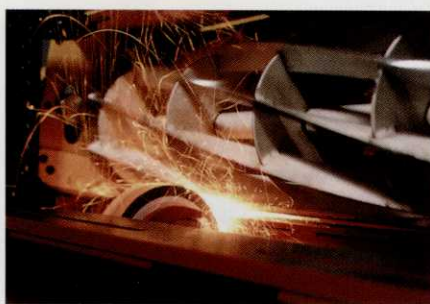
Sand and heavy topdressing eats through blades – regular maintenance is the only way to always have a healthy cut.
