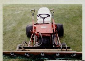
One of VanHerwynen's employees named the rake after his last name. Many of the parts/supplies were in inventory and the rake heads and muffler clamps cost about \$80. It took about 4 hours to assemble.
