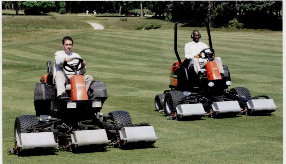
Jacobsen’s SLF-1880 has 82 inches width of cut with 18-inch Jacobson Classic XP Reels. The 18-inch reel follows ground contours without scalping.
