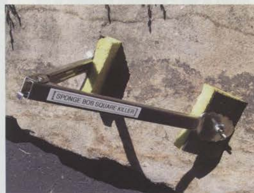
Frank Dobie, superintendent/general manager, conceived this idea at The Sharon Golf Club in Sharon Center, Ohio. Gary Bogdanski, equipment manager, modified kitchen tongs to selectively apply herbicides to kill unwanted weeds and weedgrasses in ground cover landscape beds without touching the desirable plants. Bogdanski recommends using 18-inch long kitchen tongs (or as long as possible). First, flatten each end. Then glue a 3-inch by 3-inch by 1-inch square sponge to a 3-inch by 3-inch by 1/8-inch hard rubber square and attach it to the flattened tong ends by drilling holes on each tong end and using 1/4-inch diameter stainless steel bolts and wing nuts. Spray the sponge with glyphosate herbicide or broadleaf herbicide until the sponge fully expands. Squeeze off any excess liquid so the sponges do not drip. Close the tongs on the weedgrass or weed and pull upwards. The materials cost less than $25 and the labor time is approximately 30 minutes.
