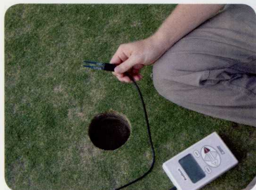
Superintendents can use devices to measure volumetric water content at different soil depths. Photo: Dara Park, Ph.D.
