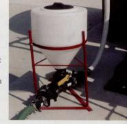
into about 600 gallons of water, which takes about 20 minutes. One control valve agitates the mixture, and another keeps the flow from being restricted into the large tank when it's in use. The agitator is used constantly as the sprayer applies chemicals or fertilizers to keep them in suspension.
