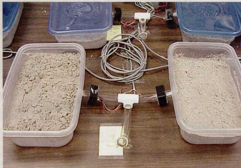
Laboratory tests with choice chambers always demonstrate a tendency for mole crickets and other turfgrass insect pests to avoid soil treated with conventional insecticides and many biological control materials. The chamber with untreated soil on the left has significant tunneling from mole cricket activity while the treated chamber on the right has very little insect activity. Photo: N.C. State University
