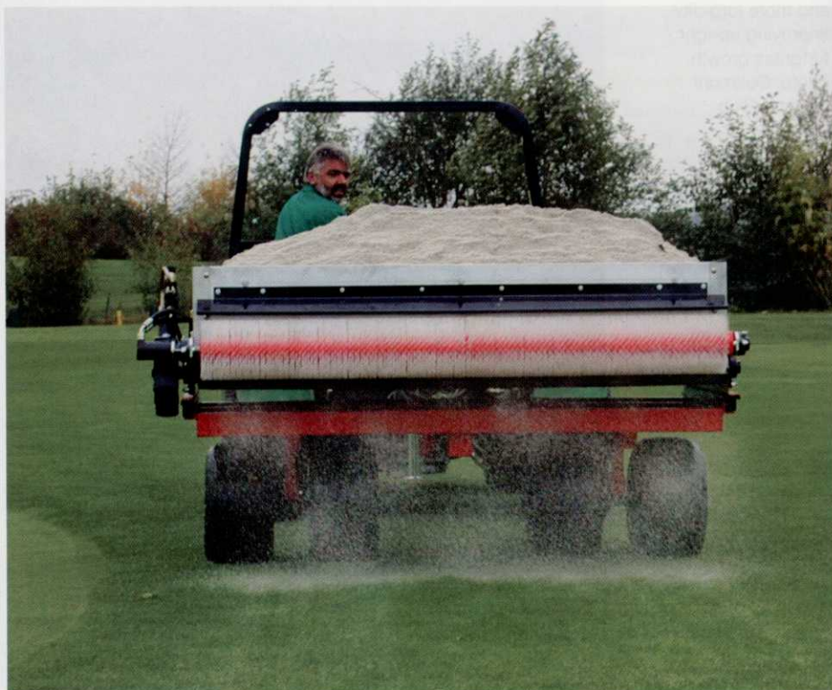
Topdressing greens with sand builds the soil system, allows for better drainage and restrains compaction. Photo: Redexim Charterhouse
