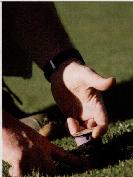
As a result of using reclaimed water, ciliated protozoa grow in the irrigation lines and can clog nozzles. Photo: Jacob Chinn
