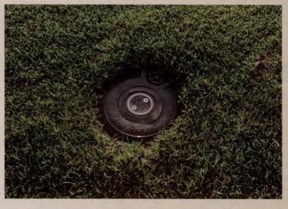
Superintendents can use rotors specifically designed for use with nonpotable water. Photo: Rain Bird
