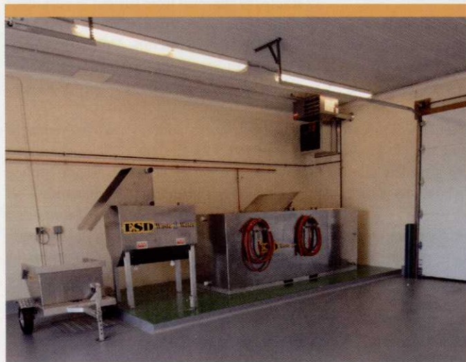
Nashawtuc’s environment management center features an ESD closed-loop wash system. Because the system is self contained, there are no leaching or rinsate issues. Photos: David Wolff
