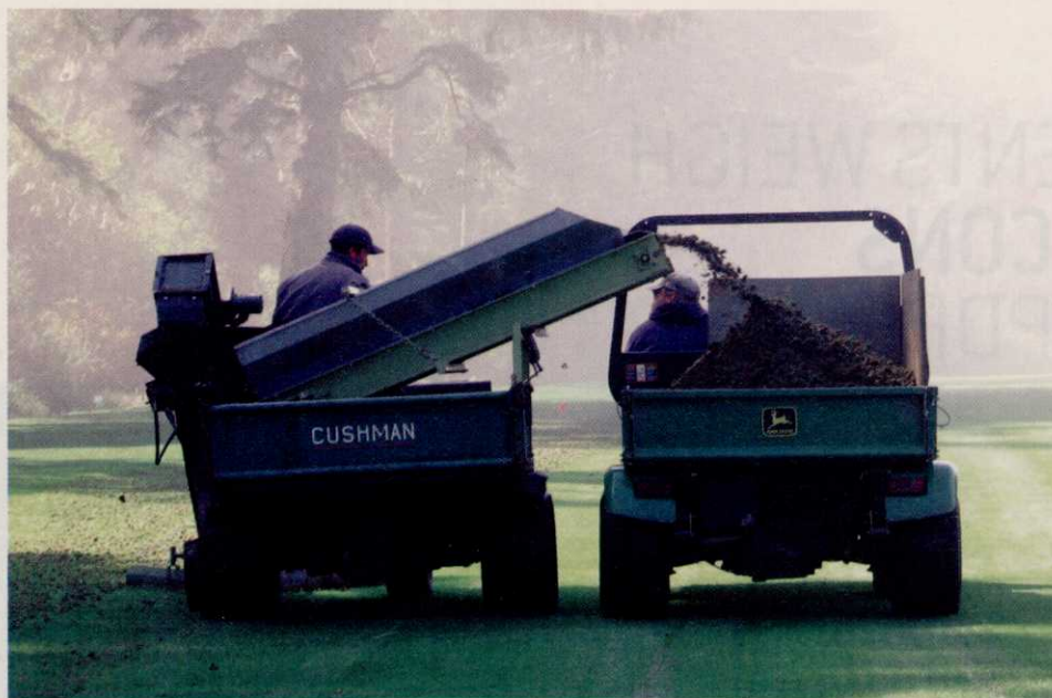
Before applying topdressing to fairways, Ryan Bancroft's crew uses a core harvester with a modified conveyor that picks up cores and transfers them to another vehicle. Photo: Salishan Spa & Golf Resort
