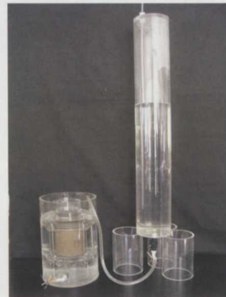
The saturation tank and permeameter was combined into a single system.
