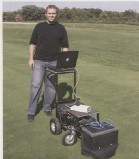
Jason Kruse uses optical sensing to identify moisture and stress in turfgrass.
