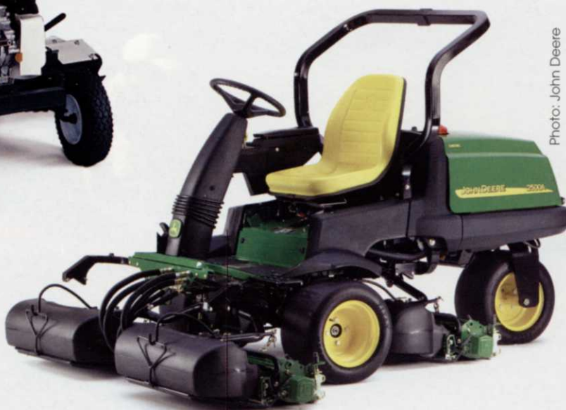
National Mower's 68 Deluxe triplex mower (top) features a 68-inch cutting width, as well as a compact and lightweight design that lets the mower maneuver through tight spaces. John Deere's 2500A triplex greens mower (right) features a new cutting unit suspension that carries the weight of the lift arms on the traction unit and not on the cutting units.
