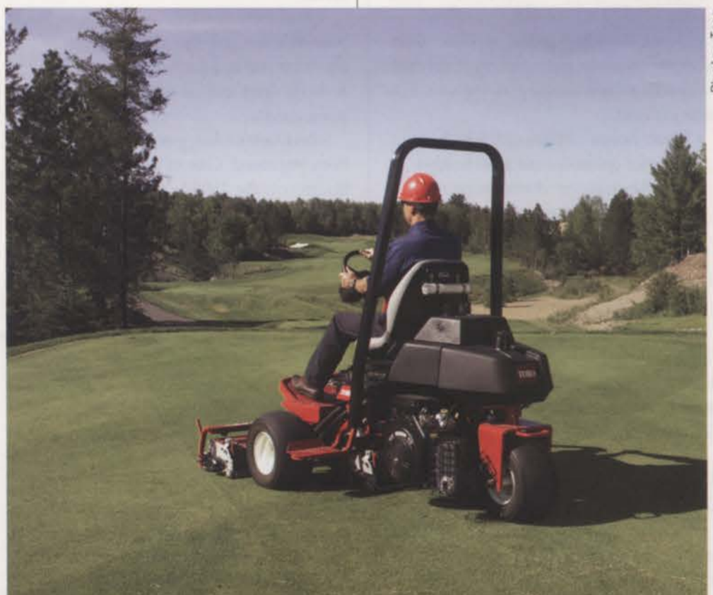
Toro's Flex 21 features a unique flexible cutting unit, specially designed for undulating greens and ultradwarf.
