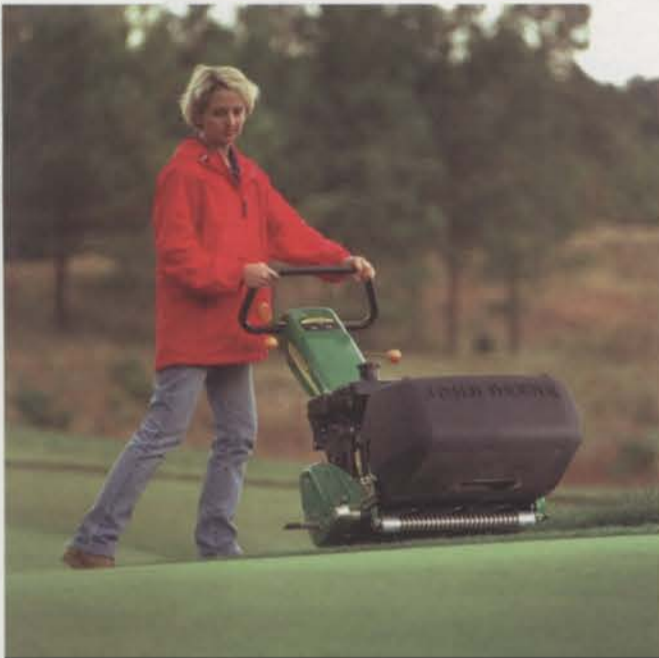
John Deere's 18-inch 180B walk mower is the ideal width for closely following green contours. The reels don't ride up and down at the ends like some flex mowers, which can result in an uneven cut.
