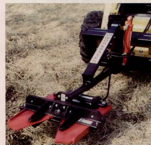
The Tree Clipper's cutting blades take out a tree.
