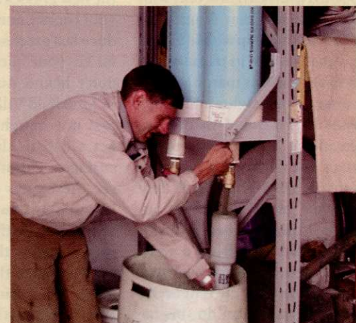
Ross' tube filler refills divot mix bottles efficiently many ways. In the photo, the tube sits in a welded square of two-inch angle iron that is
