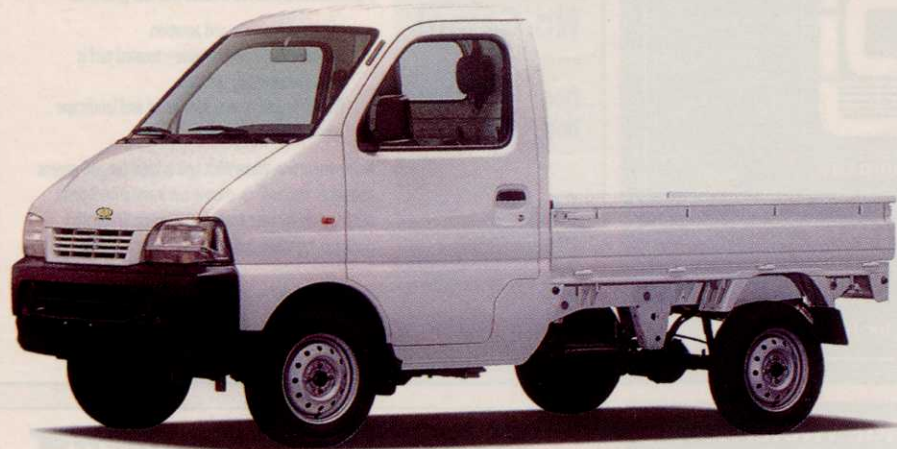
The new Micro Series features new styling and a 1300 cc, 16-valve SOHC powertrain.
