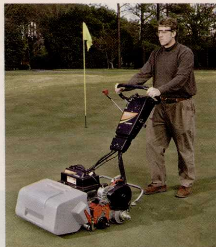
The E-walk has two 48V electric motors
