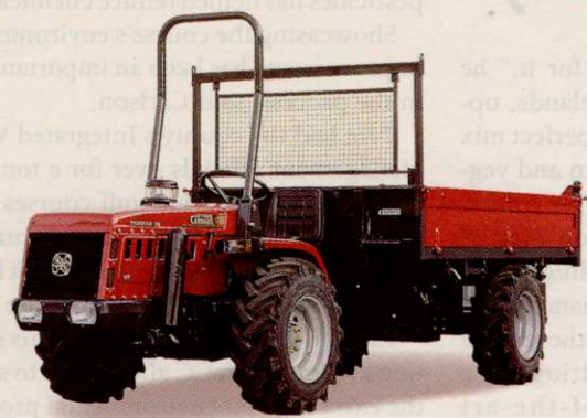
The TigreCar GST77 features three-sided hydraulic dumping
