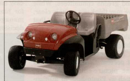
Toro added hydraulic front brakes to the 2110
