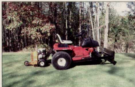
A side view of Balco's converted Billy Goat blower attached to the hydraulic lift of a Toro SandPro
