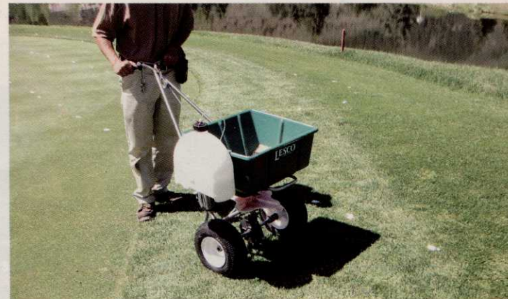
Salvarani North America's foam marking kit for walk spreaders
