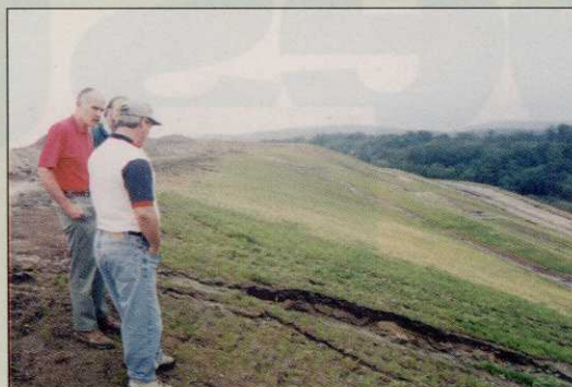
Manufactured soil, using paper fibers, helps reduce erosion. Eroded ground in foreground is normal topsoil.
