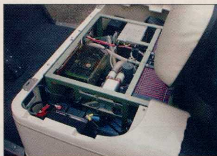
Astris Energi has retrofitted a golf car to run on hydrogen fuel-cells.
