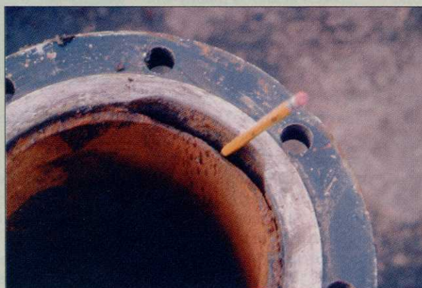
An acid-eaten section of pump station piping
