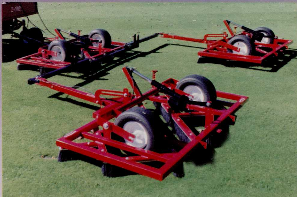
The 17' wide Triple Gang quickly grooms Fairways, stands up the grass before mowing, and disperses dew and worm casts.
