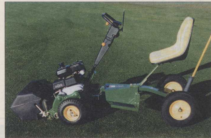
Greens mower sulky frees up turf vehicles for use by others.
