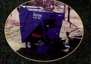
COMPACT SELF-POWERED VACUUM Rotating Rubber Finger Pick-Up 20 hp. Engine Easy Towing
