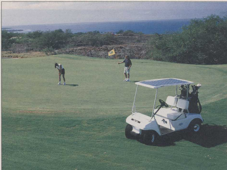
The Sun Caddy system installed on this car reduces the frequency of golf car battery recharging.
