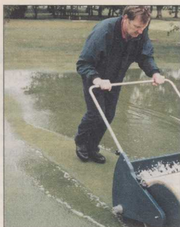
Bowdry foam roller absorbs water from turf.
