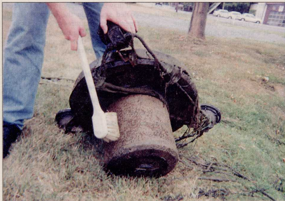
Cleaning an aerator.
