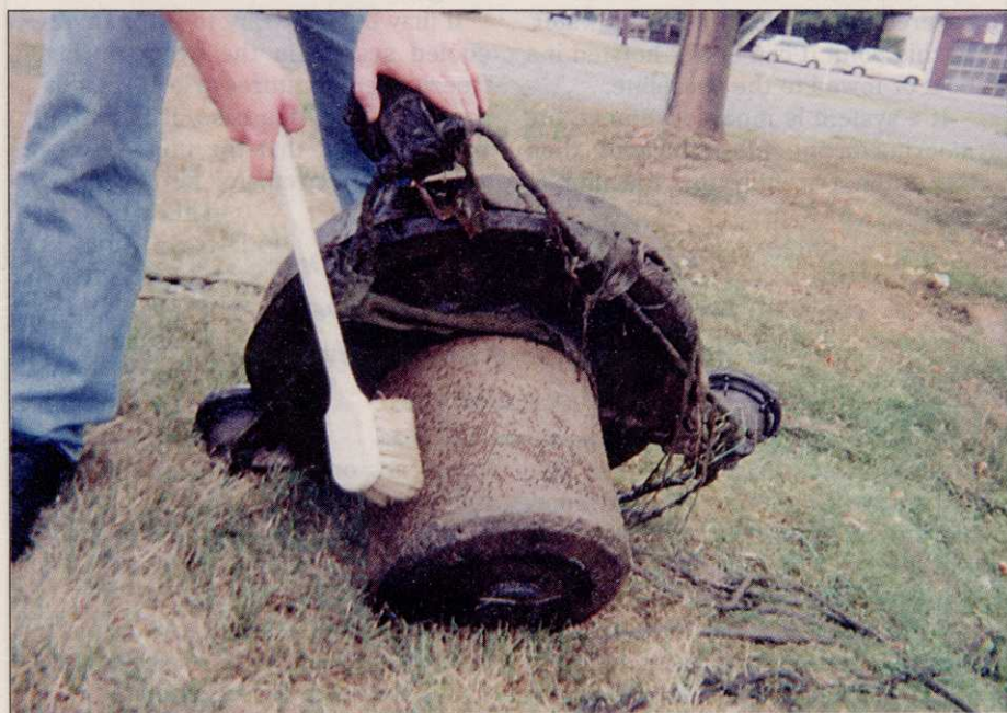
Cleaning an aerator.
