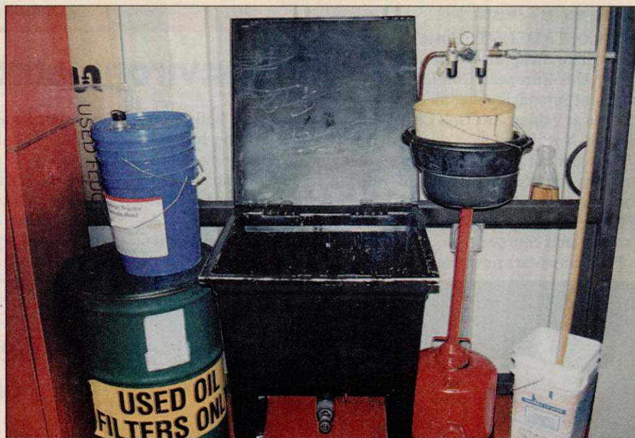
Used oils placed in a square blake container. Used oil filters are disposed of properly as well.
