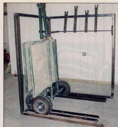
The trailer storage rack fits in a 4- by 5-foot space.
